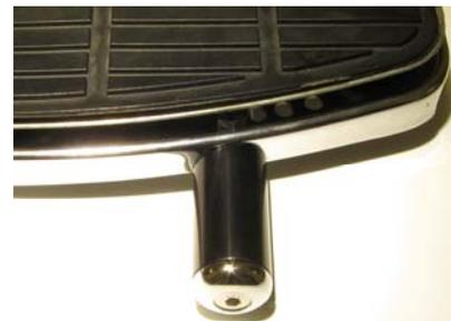
*After drilling the holes, mount the body pieces of the footrest pegs to a desired position. Mount the sleeves and end pieces. Secure the screw joint by locking.*
