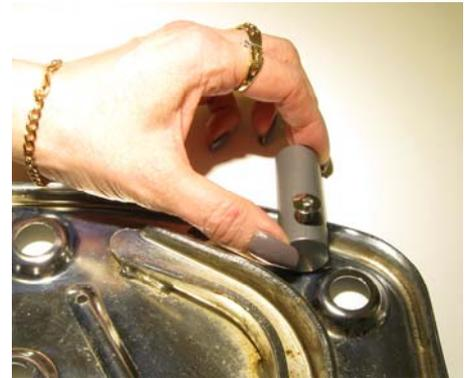
*Detach and dismantle the footboards. Take the parts out of the package and replace the ball head screws on the end piece with countersunk screws. Move the body piece a few times back and forth against the bottom of the footboard, as shown in the picture. The sharp end of the screw has now drawn the area in which you can drill one or more hole for the installation.*
