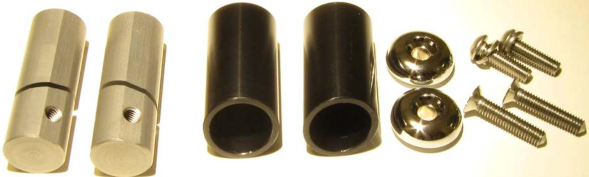
*The screws are made of stainless steel, other parts of aluminium. The body pieces on the left are anodized, the sleeves in the middle hard anodized and the end pieces chrome-plated.*
